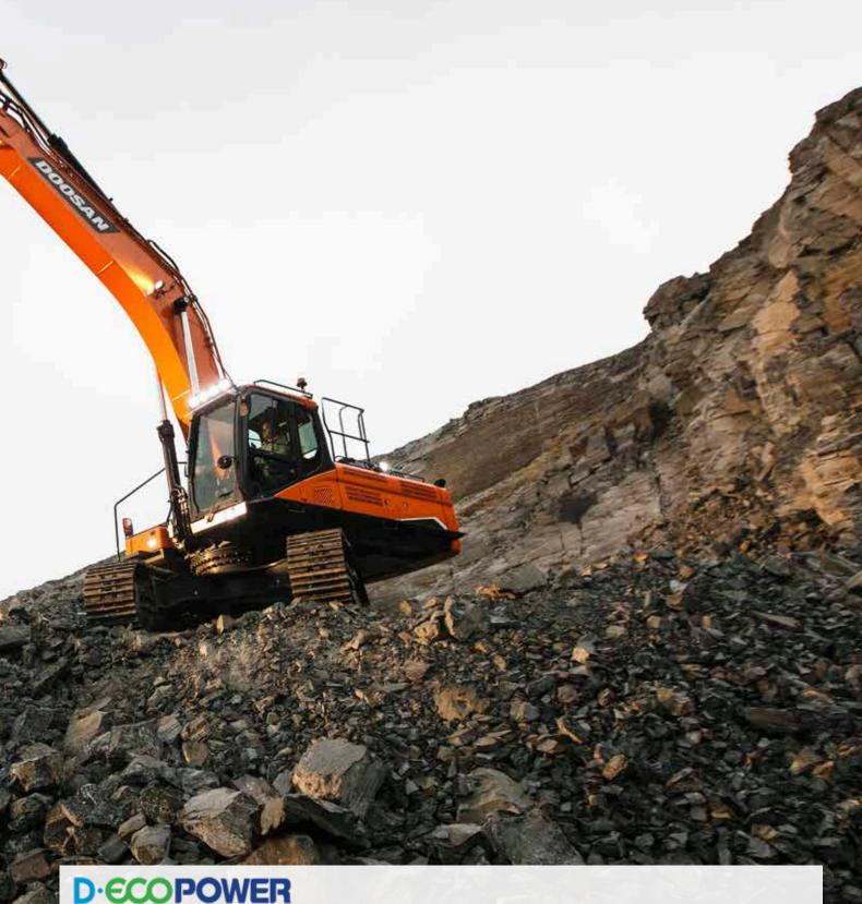
Real breakthrough technology that sets new standards in the industry: The exclusive ECO Power system improves productivity and saves fuel. A pressure-controlled pump, closed-center main control valve, and 9 sensors electronically detect and control the precise amount of hydraulic oil required to perform a task. The exact amount of oil required is metered instead of continuously forcing a fixed amount of oil through
